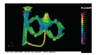
Solidification time during casting is very important in influencing the level of porosity and strength of the cast part. In this image it can be seen that a uniform cooling rate ensures proper shrinkage from feed and risers.
