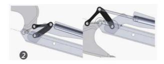
This four bar link was designed using two types of calculations; Force optimization and Link length along with angle optimization, while ensuring the full range as shown in Fig.2 was achieved.
