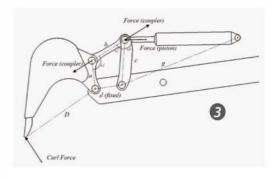
Statics equations were developed for force optimization of the mechanism according to the forces acting as shown in Fig: 3
